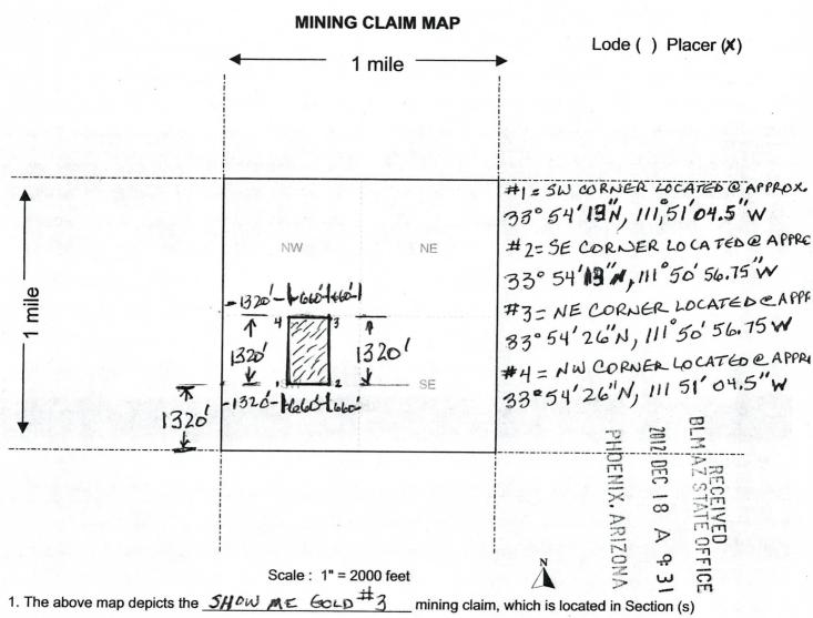
2. THE TYPE OF CORNER LOCATION MONUMENTS USED ARE 2" DIAMETER PUC PLASTIC PIPES, 4'IN LENGTH.
